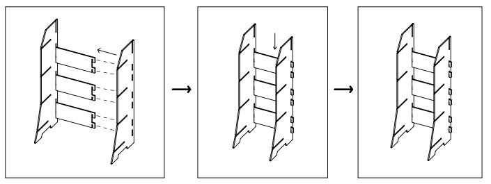
**STEP 3:** Insert the Bottom Shelf into the bottom slots on the Side Panels. *Note: If needed, using a rubber mallet (sold separately), gently tap the parts into place.*
