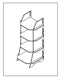
**STEP 5:** Insert the Header into the top vertical slots on both Side Panels, as shown below. *Note: If needed, using a rubber mallet (sold separately), gently tap the parts into place.*
